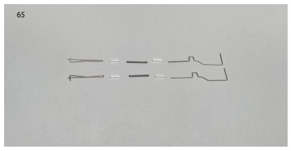
66. Use heat shrink tubing to connect the rod and the servo wire end, and apply a small amount of 502 adhesive to secure it.
