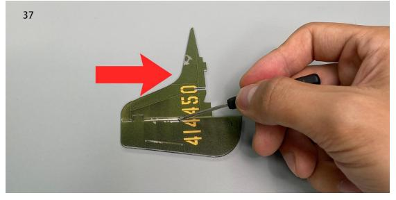
38. Install the vertical stabilizer reinforcement.
