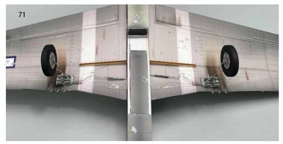
72. Bend the landing gear wires slightly towards the front of the aircraft.
