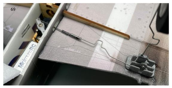
70. Install the other rod on the opposite side in the same manner, making sure the opening of the rod end clamp faces downward.
