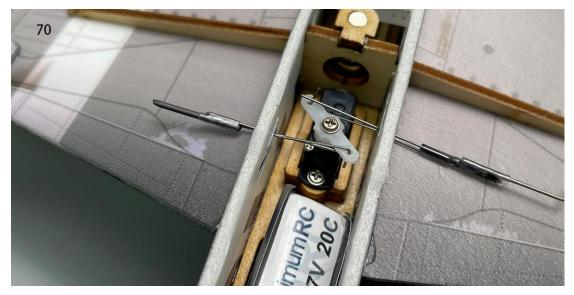
71. Adjust the length of both rods to ensure that the landing gear retracts and extends evenly into the correct position.
