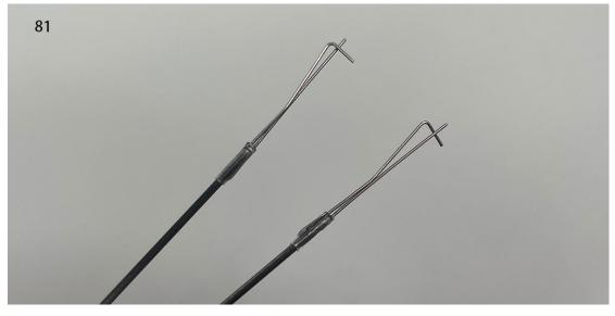
82. Install connection hooks on the tail control horns.
