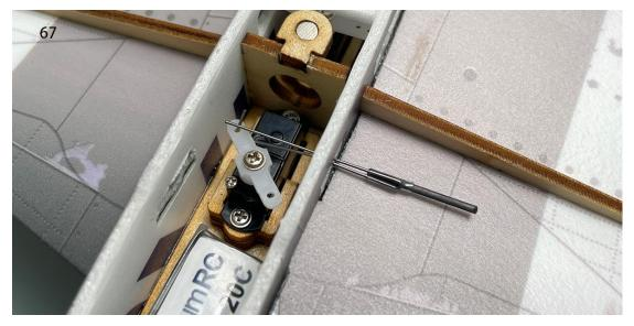
68. Install the landing gear drive rod into the groove.
