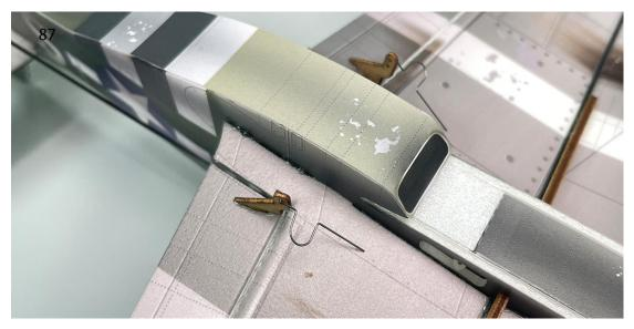
88. Insert the wire clamp heads into the fuselage and install them on the aileron servo arms.
