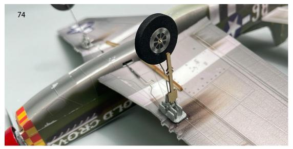
75. Install the landing gear rigid reinforcement structure in the corresponding positions.
