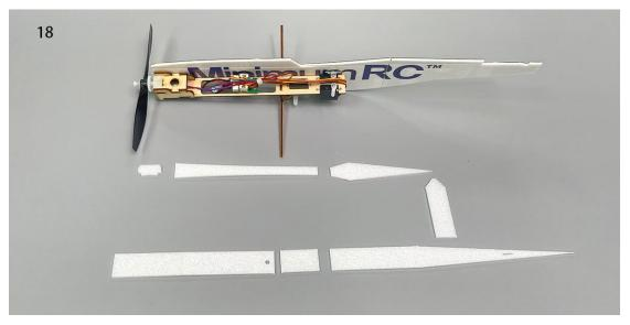
19. Press the fuselage inward along the score lines and use glue to install the bulkhead.
