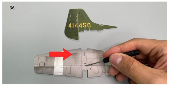
37. Use a sharp tool (screwdriver) to score through the marked lines on the bottom of the vertical stabilizer, allowing the rudder to move freely along the lines on both sides.
