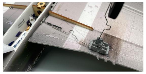
69. Use heat shrink tubing to connect the rod and the drive rod, and apply a small amount of 502 adhesive to secure it.
