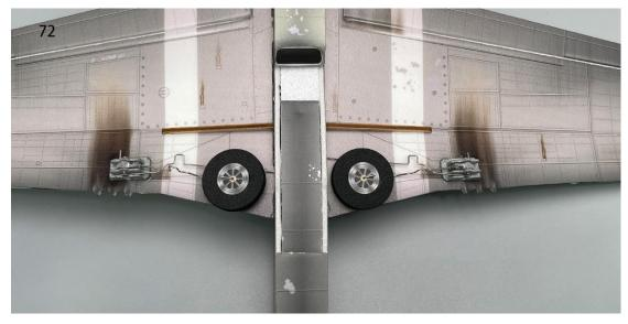
73. Adjust the landing gear wires so that they are vertical to the ground when in the open position.
