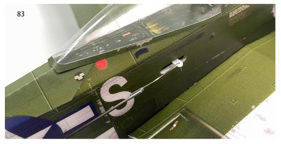
84. Trim the carbon fiber rod to the appropriate length. Use heat shrink tubing to connect the carbon fiber rod to the connection hook, then apply 502 glue for fixation.
