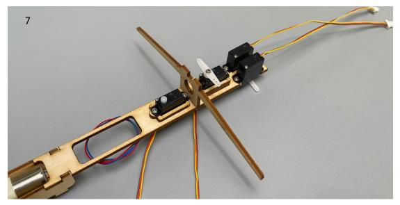
8. The landing gear servo uses a cross-shaped arm.
