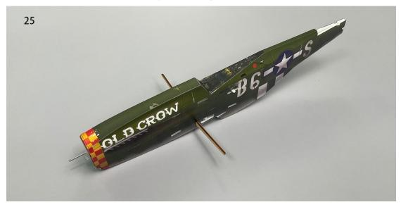
26. The front bottom plate of the fuselage can be opened forward as a battery compartment cover.
