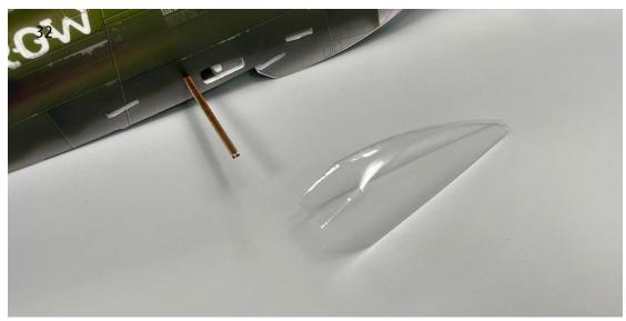
33. Install the canopy onto the fuselage at the corresponding location.
