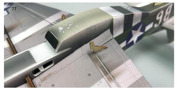
78. Install the horizontal stabilizer control horns.
