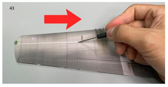
44. Use a sharp tool (screwdriver) to score along the aileron's marked line, allowing the aileron to move up and down along the line.
